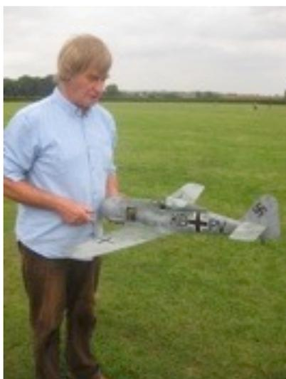
*Ivan Taylor checks out his twice-size KK Fw190. All of Ivan's models are mylar-covered and painted with acrylic. Crash-proof prop blades are attached with short lengths of trimmer nylon.*
